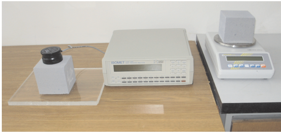
Fig. 1. ISOMET 2104 with superficial sensor
