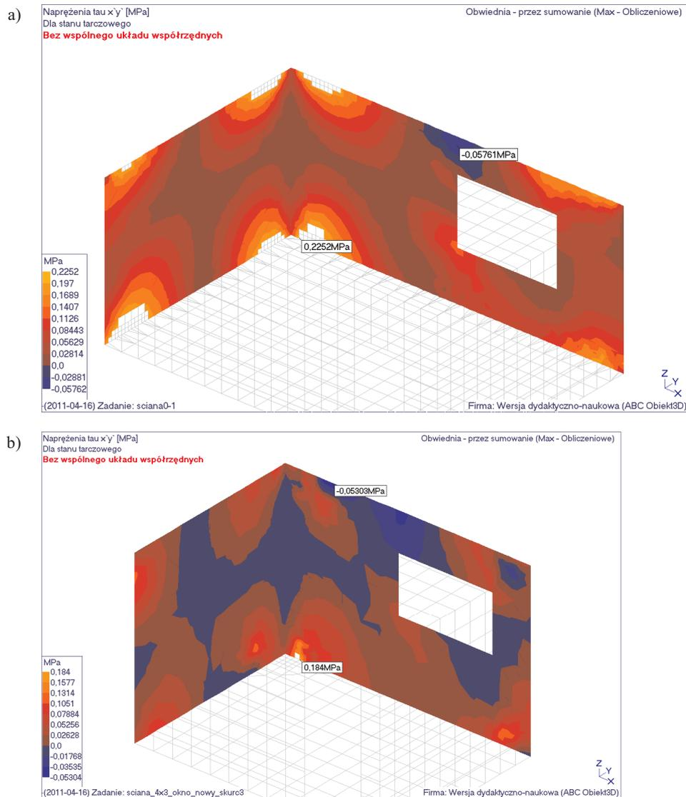
Fig. 8. Shearing stresses in walls corners: a) model I, b) model II
