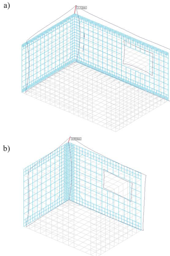
Fig. 6. Displacement of models: a) model I, b) model II
