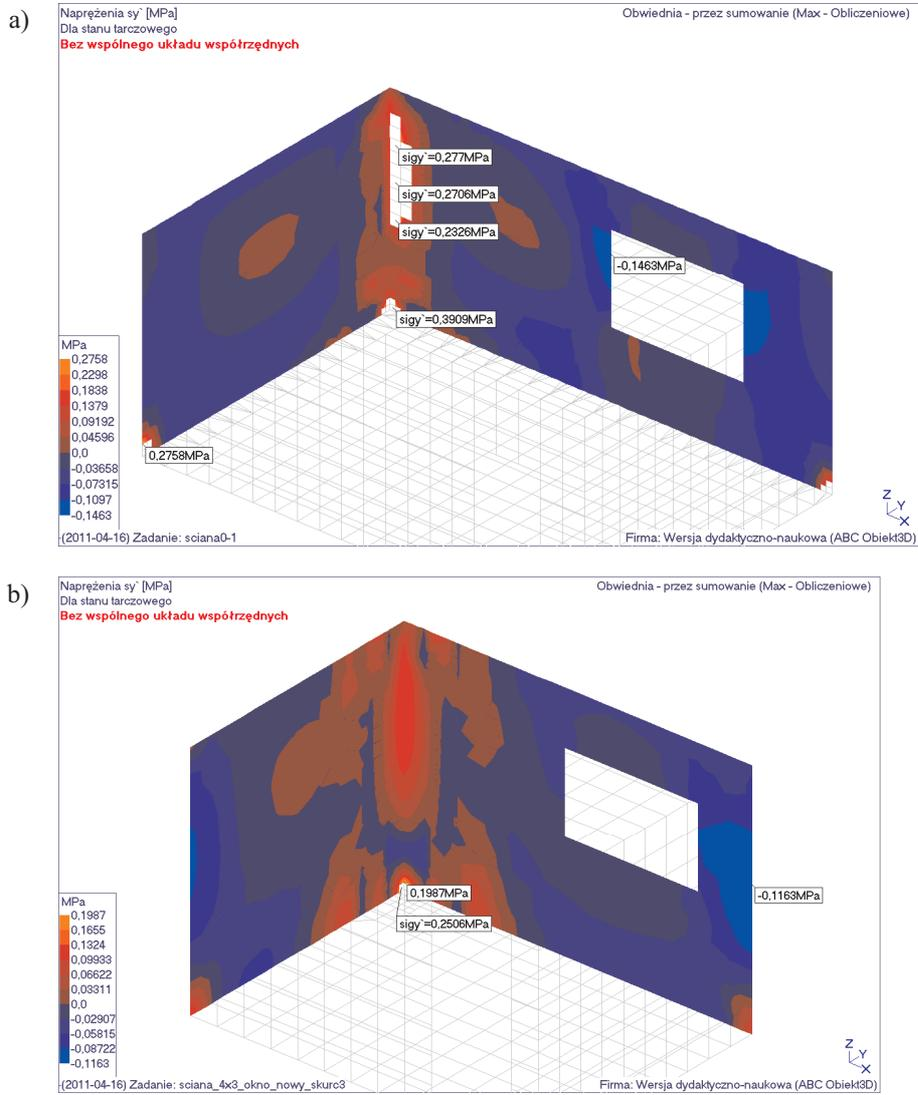
Fig. 7. Horizontal stresses in walls corners: a) model I, b) model II
