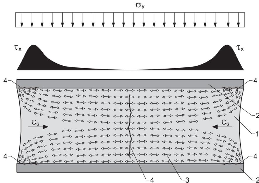
Fig. 1. Analyzed wall-ceiling model, according to [4]: 1 – wall, 2 – concrete ceiling, 3 – masonry tensile stresses, 4 – possible cracking
