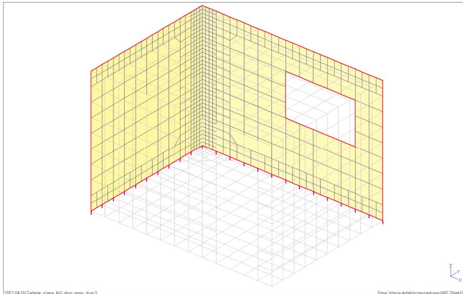
Fig. 5. Fragment of the corner of the FEM model II
