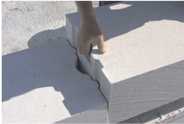
Photo 1. Material uniformity and porosity are among the most important features of ACC
